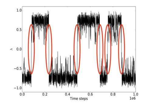
Direct molecular dynamics is, at best, an inefficient way to study a rare event; at worst, intractable. **Path** sampling methods perform a Monte Carlo simulation is the space of paths (trajectories), enabling efficient simulation of rare events by focusing the simulation effort on the transition region and reducing the simulation inside the metastable states.
